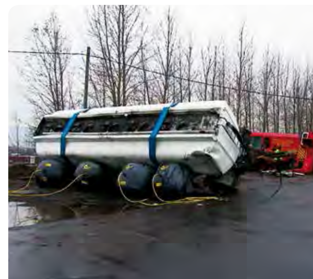
Efficient lifting of overturned vehicles.
