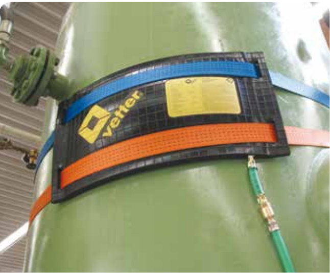
High-pressure leak sealing bag (10 bar / 145 psi)
