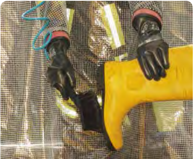
Integrated gloves for safe external cleaning
