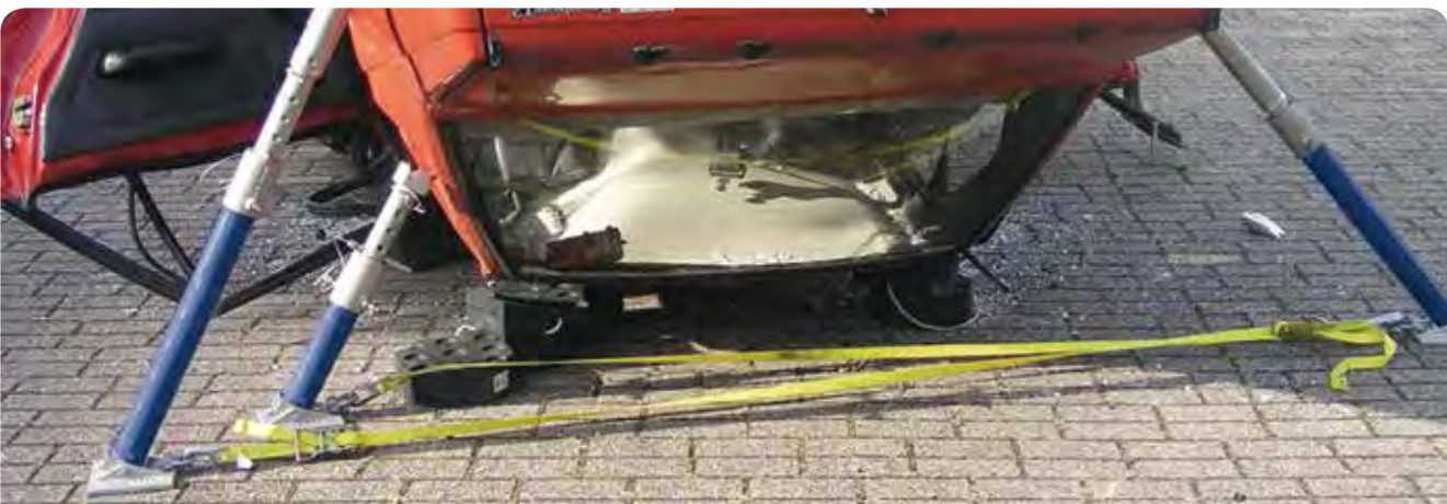
Vehicle stabilisation with ART-Lite strut.
