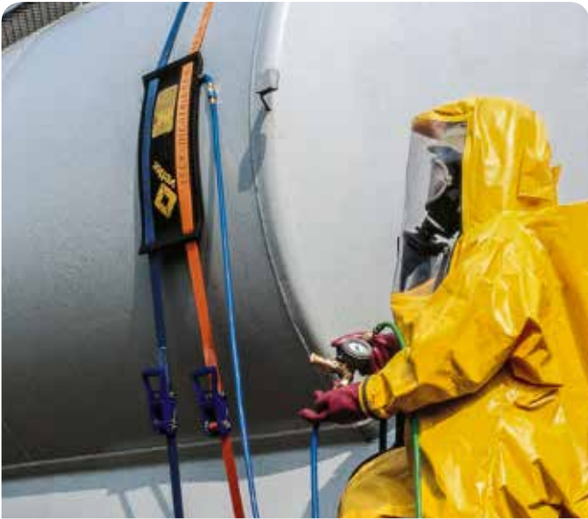
Leak sealing bag with belt slots
