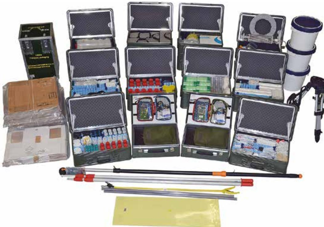
**Advanced CBRN Sampling Equipment** is a dynamic sampling kit designed for forensic and tactical sampling based on NATO sampling regulations, e.g. AEP 49, AEP 10 and AEP 66 (draft).
